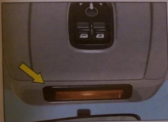
Front interior lamp Controlled by the opening of a front door or by pivoting the lens.
