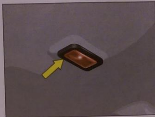
Rear interior lamp COMBI Controlled by pivoting the lens.
